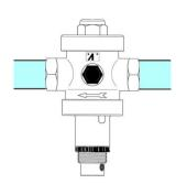
The pressure reducers DZR BRASS 143 don't get the effects, in their functioning, of gravity force; therefore they can be installed in the plant in any position:
