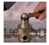
All VANTEC pressure reducers are tested before being packaged; during test they are pre-set at the outlet pressure of 3 bars; outlet pressure can be easily adjusted once the pressure reducing valve in installed on site.
